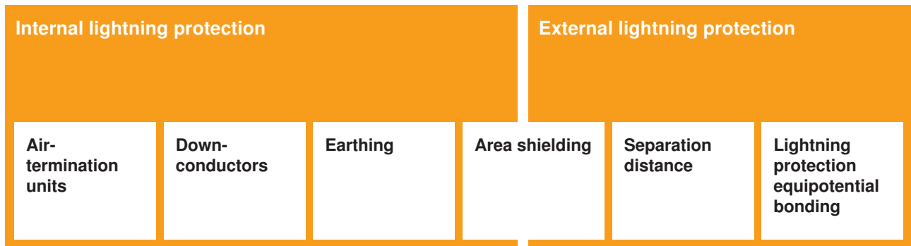
External and internal lightning protection systems
