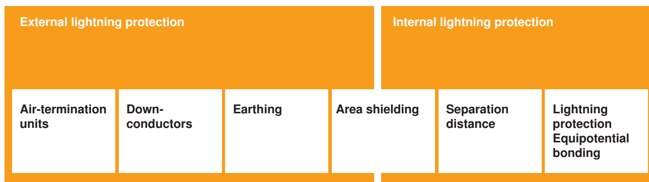
External and internal lightning protection systems
