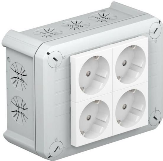
Junction box for the connection of cables indoors and in protected outdoor areas. Rectangular design with knock-out entries to the sides and knock-out entries in the bottom. Suitable for wall and ceiling mounting and on mounting panels. With the option to fasten inside and to mount via the corner domes. Cover with quick-lock, sealable with retainer and 4 Modul 45 sockets. Made from halogen-free and UV-resistant materials.
