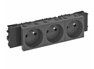
Earthing pin socket with connection to side, Triple  $0^\circ$ , with increased touch protection, with screwless terminals, 2-pin, 16 A, 250 V~, with connection terminals to IEC 60884-1, suitable for the installation in Rapid 45 device installation trunking systems.
