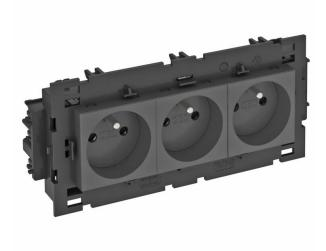
Earthing pin socket with connection to side, Triple  $0^{\circ}$ , with increased touch protection, with screwless terminals, 2-pin, 16 A, 250 V $\sim$ , with connection terminals to IEC 60884-1, suitable for the installation in Rapid 80 device installation trunking systems.
