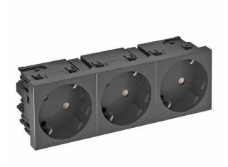
Protective contact socket triple 33°, with increased touch protection, with screwless terminals, 2-pin, 16 A, 250 V~, with connection terminals to IEC 60884-1.
