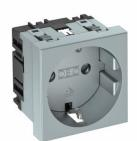
Power socket, single 0°, with increased touch protection with screwless terminals, 2-pin, 16 A, 250 V~, with connection terminals to IEC 60884-1.
