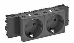
Protective contact socket with connection to side, Double 0°, with increased touch protection, with screwless terminals, 2-pin, 16 A, 250 V $\sim$ , with connection terminals to IEC 60884-1, suitable for the installation in Rapid 45 device installation trunking systems.
