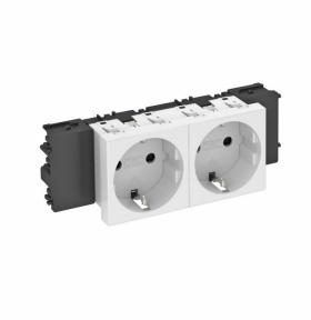
Protective contact socket with connection to side, Double 0°, with increased touch protection, with screwless terminals, 2-pin, 16 A, 250 V~, with connection terminals to IEC 60884-1, suitable for the installation in Rapid 45 device installation trunking systems.
