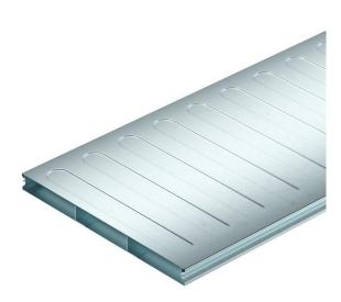
Underfloor duct (2 piece) for routing cables in screed-covered underfloor systems, according to EN 50085-2-2. Removable and continuously lockable trunking cover. With separating retainers in the trunking base. Maximum load-bearing capacity to 1.5 kN.
