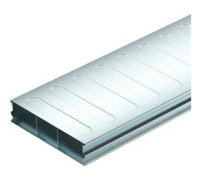
Underfloor trunking (2 piece) for routing cables in screed-covered underfloor systems, according to EN 50085-2-2. Removable and continuously lockable trunking cover. With separating retainers in the trunking base. Maximum load-bearing capacity to 1.5 kN. Only compatible with the UZD250-4/350-4 The profiled side walls offer a locking mechanism to lock the duct cover onto the
