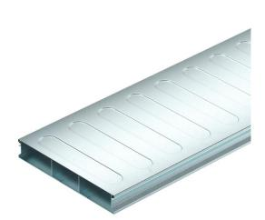
Underfloor trunking (2 piece) for routing cables in screed-covered underfloor systems, according to EN 50085-2-2. Removable and continuously lockable trunking cover. With separating retainers in the trunking base. Maximum load-bearing capacity to 1.5 kN.
