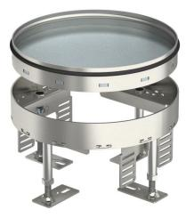
Round, "blank", heavy-duty cassette of nominal size R4 for the creation of an inspection opening in trunking systems, raised and cavity floors, in dry or wet-care floors for indoor use. Load class 2 to 20 kN. Only suitable for smooth floor coverings.
