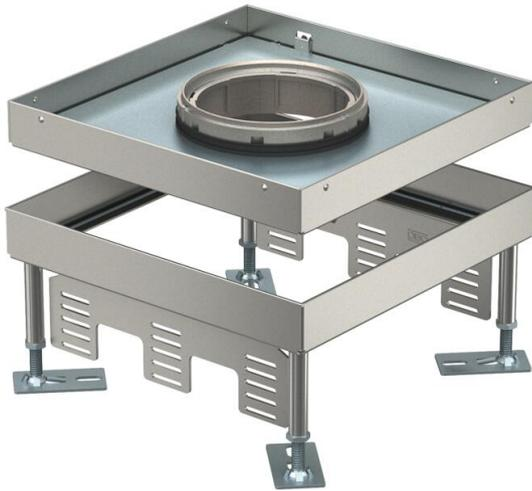
Height-adjustable heavy-duty cassette for tube bodies of nominal size 9 for the installation of devices in duct systems, raised and cavity floors in interior dry or wet-care floors. Load class 1 to 10 kN.
