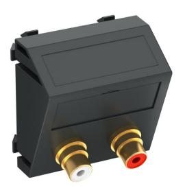
Multimedia support with two cinch connection sockets for audio R/L, slanting cable outlet, with labelling panel, two cinch couplings (RCA), socket-socket version, colour coding red/white. Support plate with locking fastening, suitable for horizontal and vertical installation in the system environment.
