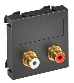
Multimedia support with two cinch connection sockets for audio R/L, straight cable outlet, with labelling panel, two cinch couplings (RCA), socket-socket version, colour coding red/white. Support plate with locking fastening, suitable for horizontal and vertical installation in the system environment.
