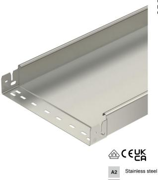
Unperforated cable tray with integrated quick fastening system. The usable length of the cable tray is 3,000 mm. Continuous equipotential bonding is guaranteed without additional components.
