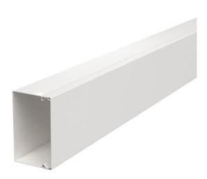
Duct cover and base with base perforation. Equipotential bonding is guaranteed between the cover and the base without any additional aids. The LKM cable duct, type LKM 60100, has been tested for the maintenance of electrical function as a routing system according to DIN 4102 Part 12. Please note the cable types tested in the BSS fire protection systems division!
