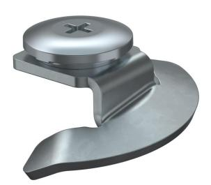
Turn buckle for additional installation or installation at a later date. Single-sided turn buckle. Use for cover widths of 100–600 mm. Depending on the cover version, dimension B varies as follows: DRL/ DRLU = 27 mm
