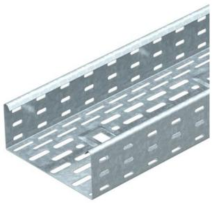
DKS 85 = perforated cable tray system with 85 mm side height. Permeable cable tray system to VdS guideline 2092 with 30% hole surface for use under sprinkler systems.
