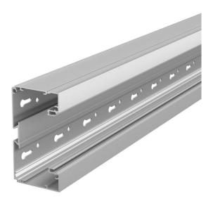
Device installation trunking with base perforation for direct wall mounting or mounting on panels. Other RAL colours can be supplied on request. The visible surfaces of the painted device installation trunking are laminated. The cover must be ordered separately.
