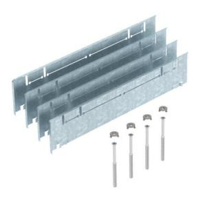
Height compensation set for underfloor boxes UZD350-3 with a construction height of 70 to 125 mm, consisting of four fall plates, four height adjustment screws and four rotary locks.
