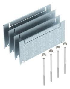
Height compensation set for underfloor boxes UZD250-3 and UGD250-3 with a construction height of 70 to 125 mm for construction stacking of the UZD/UGD to a height of 115-170 mm, consisting of four fall plates, four height adjustment screws and four rotary locks.
