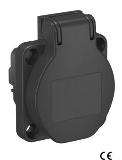
Protective contact extension socket  $0^{\circ}$  with hinged cover, with screwless terminals, 2-pin, 16 A, 250 V~, with connection terminals to IEC 60884-1. Protection rating: IP44.
