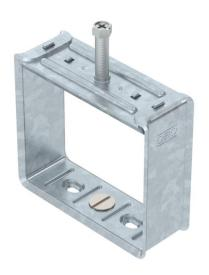
Clip and bolt made of hot-dip galvanised steel, countersunk head bolt made of rustproof stainless steel, slide nut made of electrogalvanised stainless steel. Stainless steel version: clip and screw made of hot-dip galvanised steel, slide nut, type 5019, made of rust-proof stainless steel.
